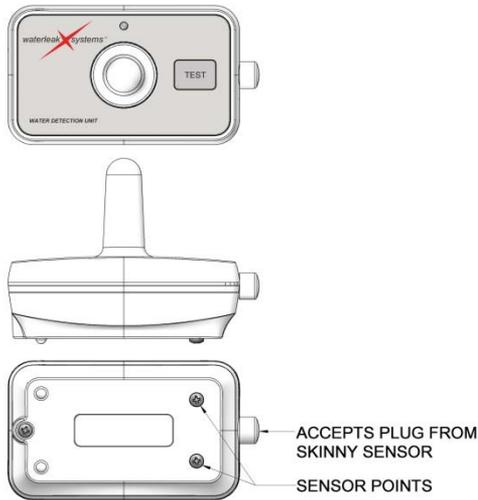
REMOVE 3 SCREWS TO INSTALL BATTERIES
